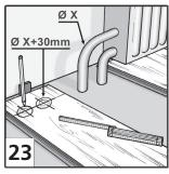
For heating-radiator pipes, holes that are drilled 3 cm/1.2" larger than the pipe diameter must be avoided. A "fitting piece" should be cut out, glued, fitted in and fixed in place with a wedge until the glue has dried. Then cover the recesses with a radiator-sleeve **[23, 24, 25]**.
