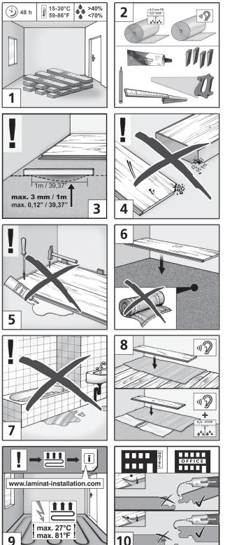
**Preparation:** Please store the packets 48 hours prior to installation under the same climatic conditions (temperature and moisture) as the actual installation process [1]. Important pre-condition for proper fitting and long-term durability of the laminated flooring is a room temperature of ca. 20°C/68°F and a relative humidity of around 50 – 70%.
