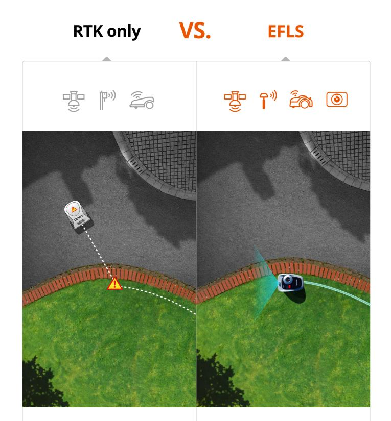
When the satellite signal is weak, the robotic mower might stop working or navigate outside the boundary.
