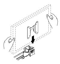
Slide the monitor (with VESA plate) onto the arm and make sure it "clicks" securely into position.
