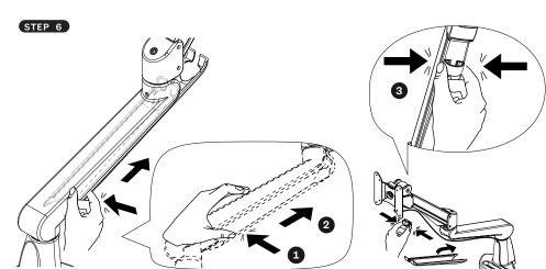
Unattach the cable collector and route the cables through. Once satisfied, re-attach the collector back into place. Proceed by continuing the routing through the cable clip.
