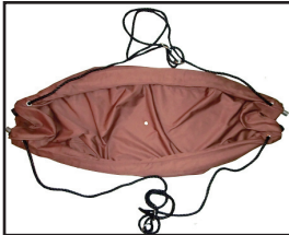
9. After the 4 rope ends are pulled, make the swing body smooth again before the triangle ends assembly.
