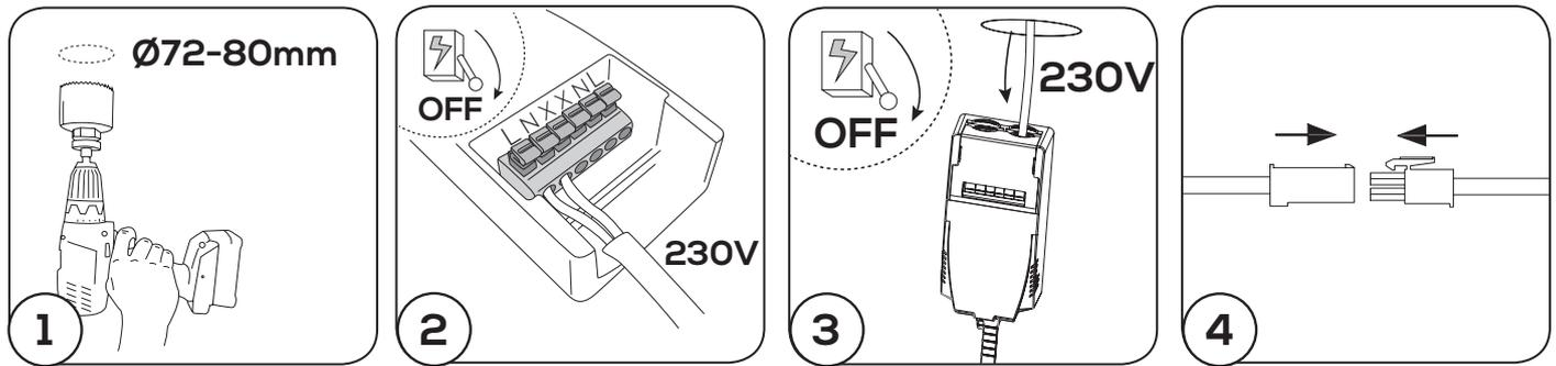
**Switch off the power before installation!**
