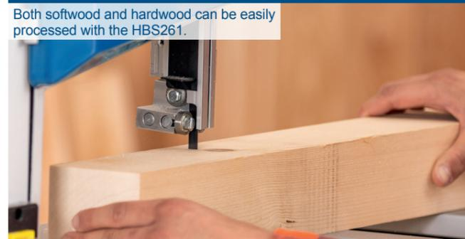
Even delicate work can be effortlessly implemented, thanks to the different saw band widths.
