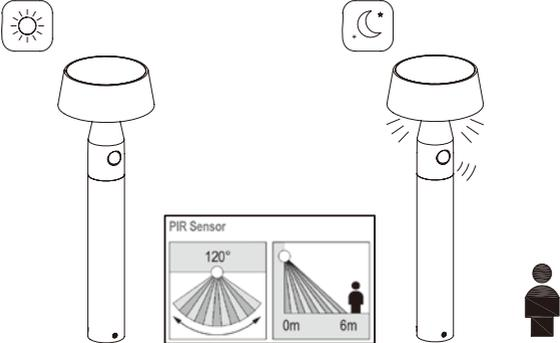
**BRT:** (1) The light will constantly output 65lumen when the day light is less than 30LUX.
