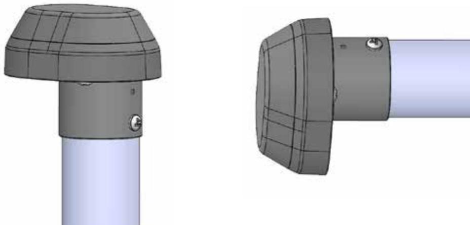
*Verify that the toilet is receiving power by checking that air is exiting the ventilation outlet.*
