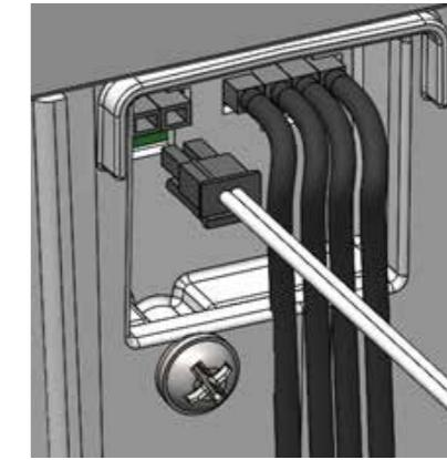
The toilet must be connected to a power source. The toilet comes with a power adapter for 110–240 V and a 12 V battery cable. Regardless of the power source, the chord must be connected to the back of the toilet, at the marked input in the picture above. Make sure that the plug is properly connected.
