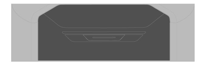
The status LED displays an inwards running pattern when the extra battery is powering off.
