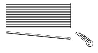
For cutting in length ways a craft knife can be used to cut through the felt.
