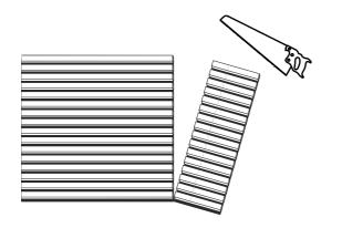
For cutting in width ways we recommend a sharp saw to cut through the slats and felt.
