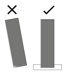
Do not put the wall panel directly on floor, the MDF veneer will be broken if it touches something hard. Put the wall panel on cartons or some soft pad.
