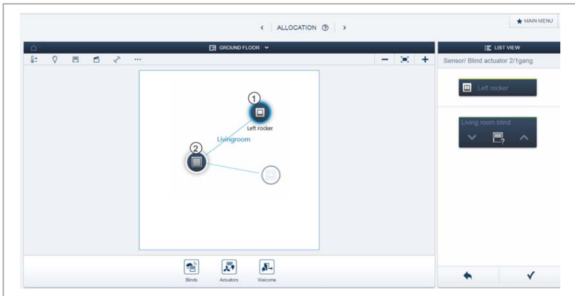
Fig. 21: Linking an actuator with an additional sensor
