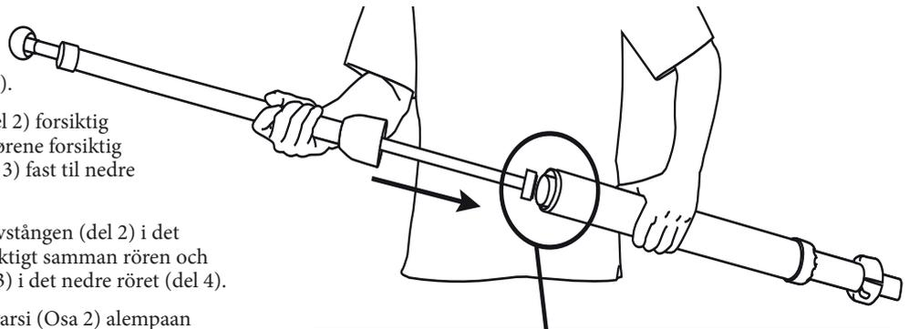
Note: Head of Lower Piston Rod fits snugly into Lower Tube. Some pressure may be needed to insert.
