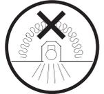
Must not be installed directly in insulation
