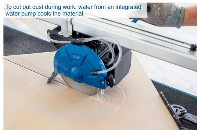
To cut out dust during work, water from an integrated water pump cools the material.
