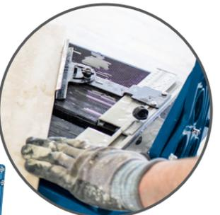
Angular stop from -45° to +45° for mitre cuts
