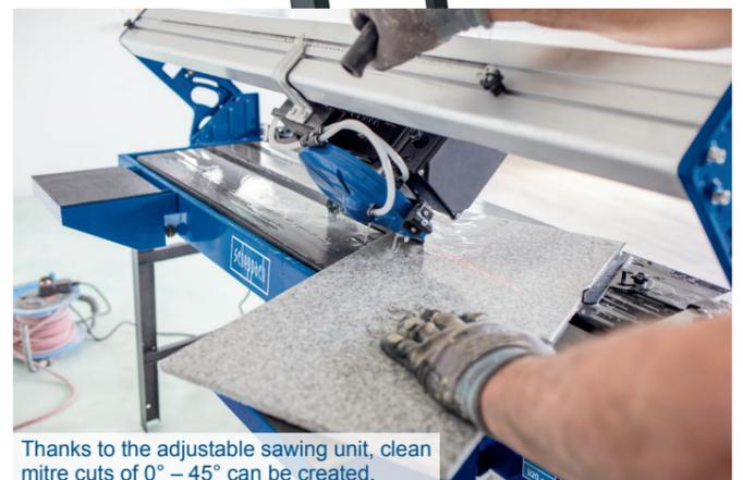
Thanks to the adjustable sawing unit, clean mitre cuts of 0° - 45° can be created.
