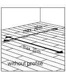
Measure the room to become a balanced lay out. By measuring, you will be able to determine if the first row needs to be cut. The first and last row should not be less than 5 cm wide.
