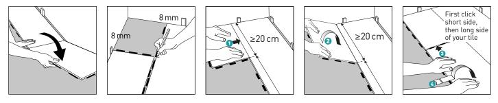
Always ensure that the short end joints will be staggered minimum 20 cm (= 2 click elements) when you start the next row. Use the leftover piece from the previous row as the first piece of the next row, provided that this piece is at least 20 cm. In order to find a connection with the locking tabs of the previous row, it may be necessary to cut off an extra part of the leftover piece.
