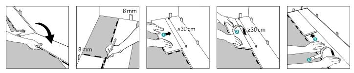
Always ensure that the short end joints will be staggered minimum 30 cm (= 3 click elements) when you start the next row. Use the leftover piece from the previous row as the first piece of the next row, provided that this piece is at least 30 cm. In order to find a connection with the locking tabs of the previous row, it may be necessary to cut off an extra part of the leftover piece.
