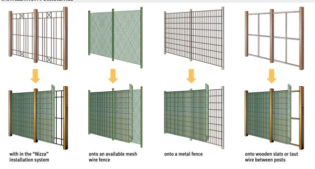
Installed quickly and securely with the VIDEX wire straps or plastic fasteners
