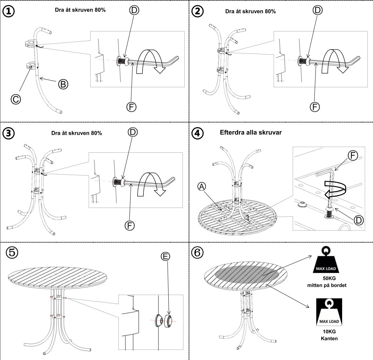
Do not tighten screws until all screws have been assembled !
