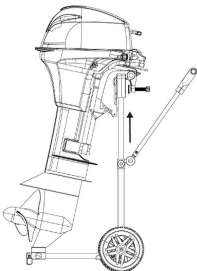
Step 4: Tighten the knob of the tube with the bracket to fix it in position.
