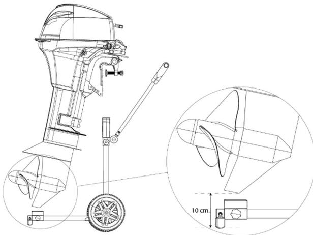
Step 2: Tilt the outboard engine so that it is straight above the bracket.
