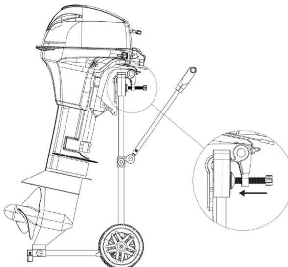
Step 5: Hand tighten the clamp screws of the outboard engine to the trolley bracket.
