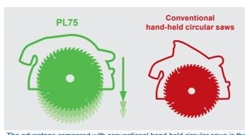
The advantage compared with conventional hand-held circular saws is the plunge function. Using this function, specific demands that require plunging the saw blade into the material can be implemented without problems.
