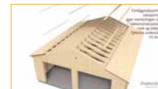
Monter undertak / rupanel
