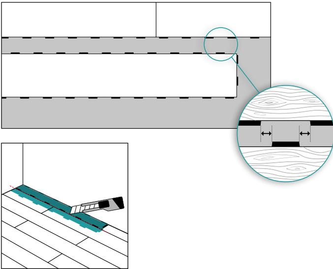
The click elements of the new row, need to be positioned, exactly in the middle of two locks of the previous row.
