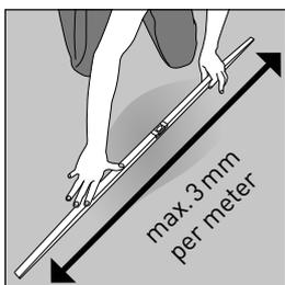
Pure Click can be installed on top of concrete, tiles, wood and most existing hard surface floor coverings, provided that the subfloor is smooth, dry and clean.
