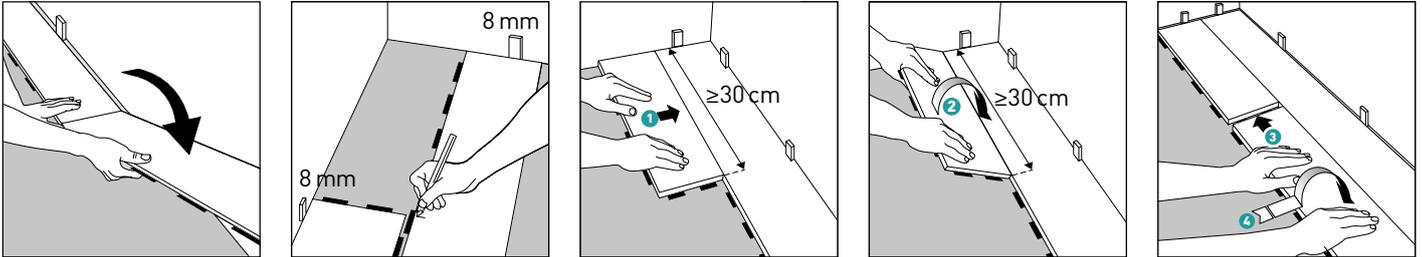
Always ensure that the short end joints will be staggered minimum 30 cm (= 3 click elements) when you start the next row. Use the leftover piece from the previous row as the first piece of the next row, provided that this piece is at least 30 cm. In order to find a connection with the locking tabs of the previous row, it may be necessary to cut off an extra part of the leftover piece.
