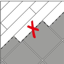
Never place the joints, where two planks are clicked together, parallel on top of the existing joints of the old tile subfloor.
