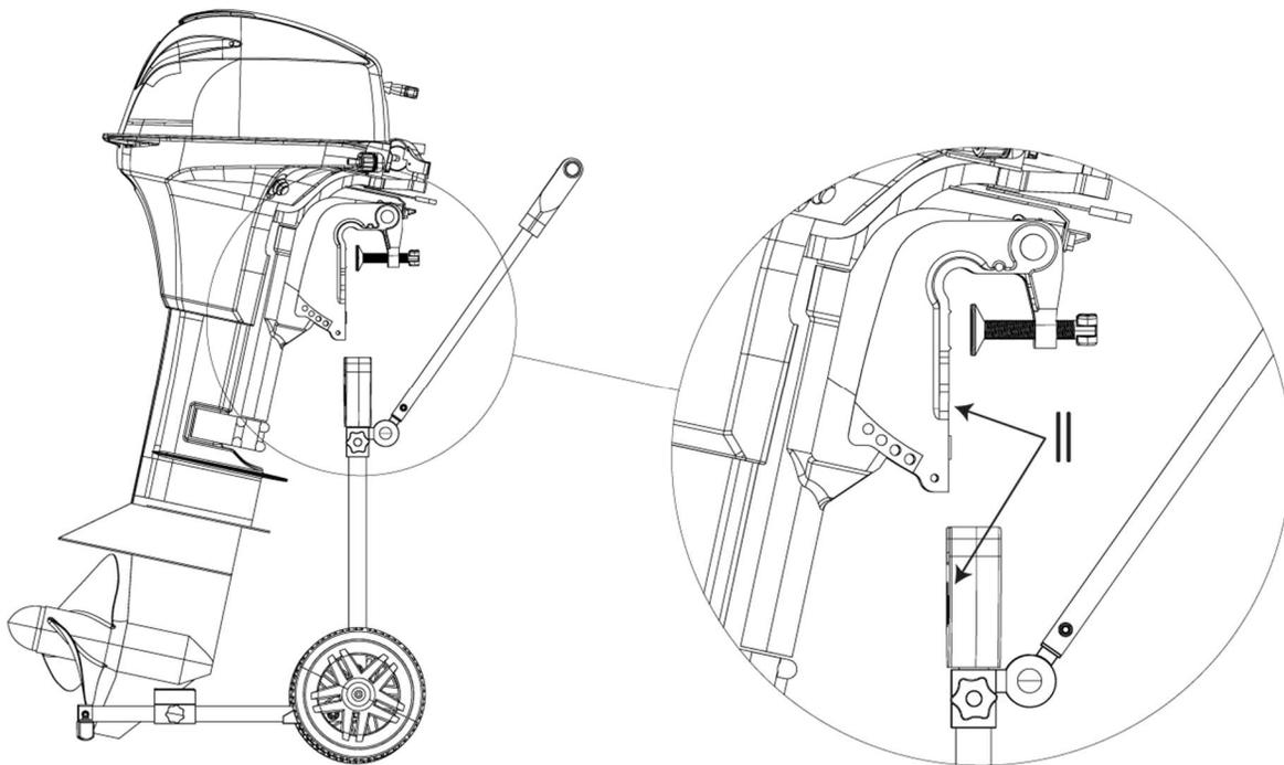
Step 4. Measure the horizontal distance between the bracket and the end of the engine tail.
