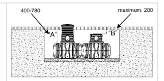
The tanks may not be installed in areas used by passenger cars.
