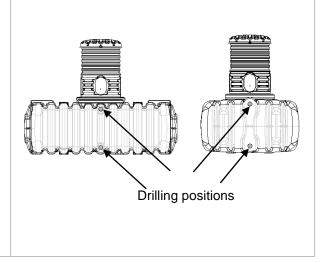
longitudinal or the transverse sides in the installation pit
