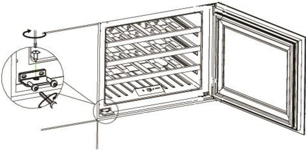
1. Put the wine cooler into the cabinet, then adjust the wine cooler to make it steady. Open the door, take out the fixing plate (1 pcs) , inner Hexagon Screws ((2 pcs) , inner Hexagon Screwdriver (1 pcs), selftapping screws (1 pcs) from the accessory bag.
